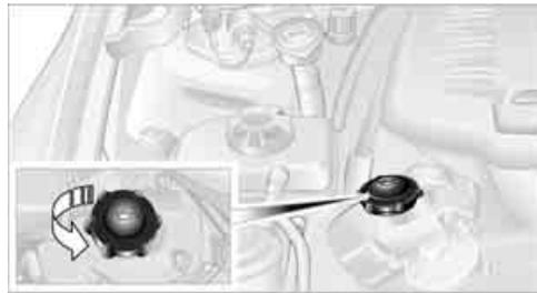
Do not add 1 US quart/1 liter of engine oil until the display shows an oil level measurement of "+1qt" or "+1l".
