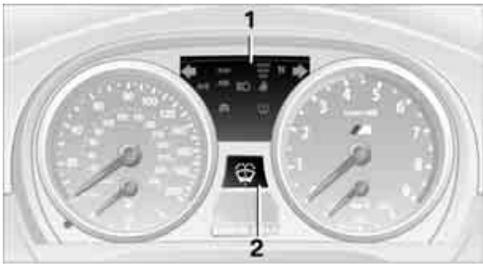
Indicator and warning lamps appear in the display area. See the table for information on causes and how to react. Note whether a lamp comes on alone or in combination with another. Some lamps can light up in different colors. Corresponding distinctions are made in the text.
