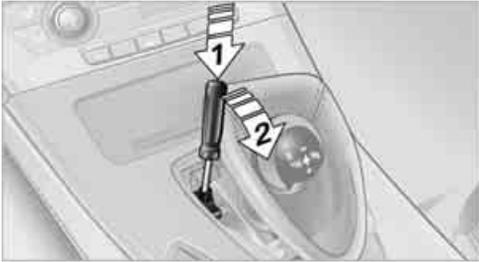
5. Pull the screwdriver back all the way, arrow 2. The parking lock is released.
