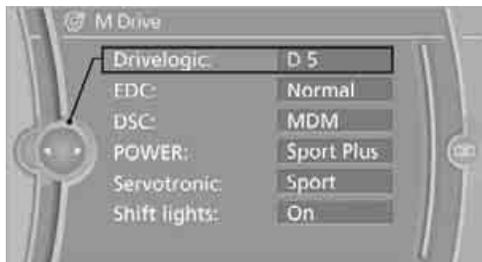
4. Turn the controller to set drive mode or sequential mode.
