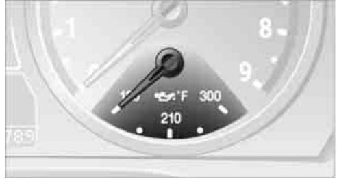
When the engine is at normal operating temperature, the engine oil temperature is between approx. 175 °F / 80 °C and approx. 250 °F / 120 °C.
