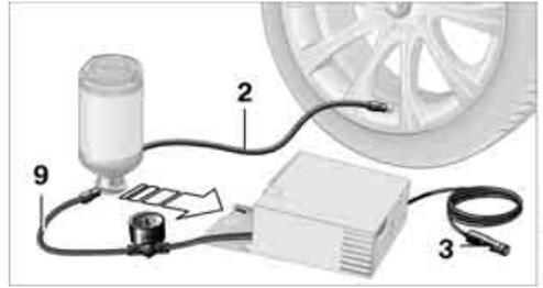
5. Unscrew the dust cap from the valve of the defective wheel and screw the filling hose **2** of the sealant bottle onto the valve.
