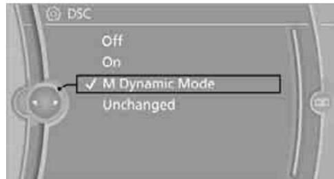
"Unchanged" retains the current setting created outside of M Drive, e.g. via the buttons in the center console.
