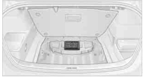
The M Mobility System is located in the cargo area under the floor board.
