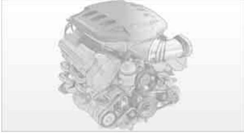
The high-speed V8 engine uses its 244 cu in/ 4 liters of displacement to produce a maximum output of 414 hp and a maximum torque of 295 lb ft/400 Nm. Its spontaneous response results in a very wide effective rpm range. The maximum engine speed is 8,400 rpm and is electronically regulated. Because of the powerful engine dynamics, the maximum engine speed is limited to 7,000 rpm when the vehicle is stationary.
