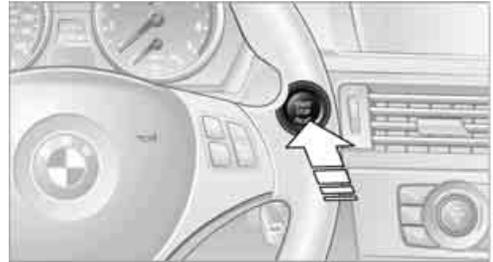
The engine starts with the selector level in any position. Driving off: with the engine running, move the selector level from the middle position ● in the desired direction.
