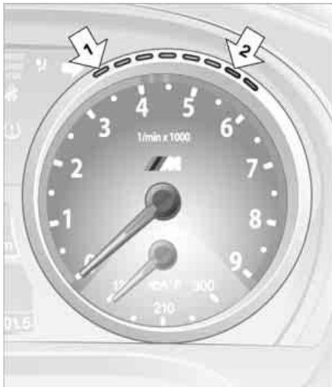
1. As the vehicle approaches its maximum engine speed, the yellow LEDs 1 light up consecutively to indicate the impending shift point.
