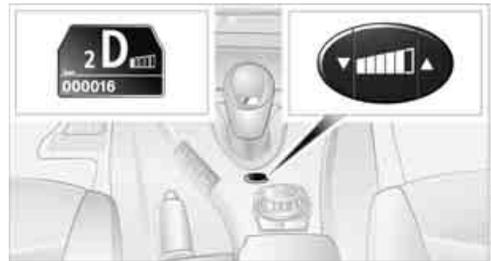
Press the button repeatedly until the desired drive program is displayed in the instrument cluster, refer to page 27.
