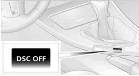
Press the DSC OFF button for longer than approx. 1 second until the DSC indicator lamps in the instrument cluster light up. DSC and M Dynamic Mode are both deactivated. Stabilizing and drive-output promoting actions are no longer executed.
