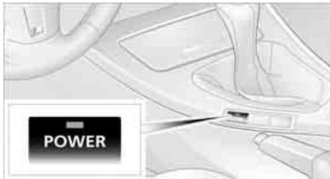
Press the POWER button to switch between the "Normal" and "Sport" programs.
