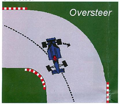
Oversteer is when the rear wheels are carving a larger arc than the front wheels or the intended line of the turn. Rear "slip angles" exceed those of the front tires. This is often described as a "loose" condition, as the car feels like it may swap ends, or be "twitchy."
