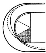
**Late Apex.** Apexing late is always the safest line and the one we teach in this class. When learning a new track, or turn, you should always start late and then slowly bring the apex back towards the mid apex; that is until you use the entire track and none of the wall on the exit. Notice how much track is not being used on the exit of the turn.
