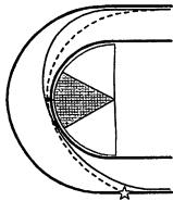
**Mid Apex.** Apexing somewhere through the middle of the turn, in this case, can make you or break you. A "later" mid apex will give you maximum use of the track width needed for the greatest exit speed. Apexing a few feet sooner will either scrub off exit speed or door paint on the wall.
