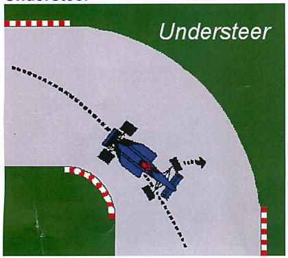
Understeer is when the front wheels are carving a larger arc than the rear wheels. This is often described as "push" or "pushing" - as the front end feels like it is plowing off of a corner.
