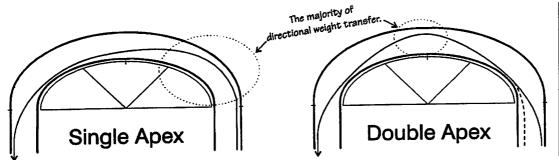
A single apex has a larger radius enabling a smoother weight transfer of the car over a larger turning track area. The braking and the majority of the turning is done in the first third of the corner allowing the driver to accelerate sooner than a double apex. When you are trying to change the direction of a 3000 lb. Car, you want the largest area possible with the least amount of angle
