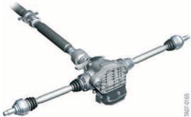
71 - E92 M3 Axle drive with output shafts
