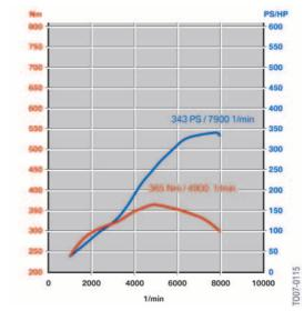
15 - E92 M3: S65B40O0 Power and Torque Curve
