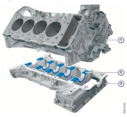
33 - S65B40 Engine block with bedplate construction
