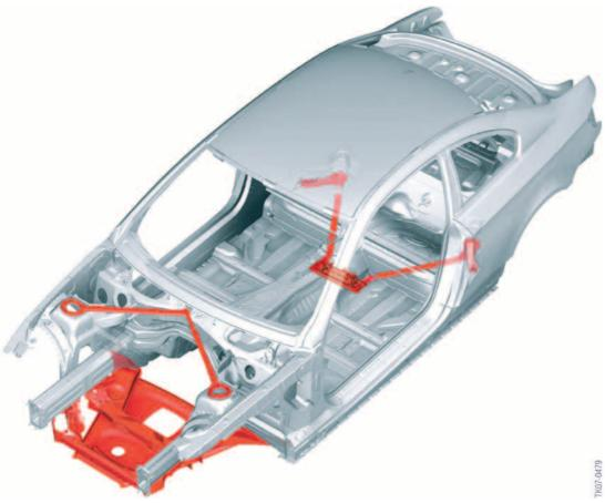
4 - E92 M3 Overview of additional bolted-on reinforcements
