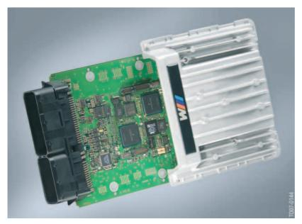
55 - E92 M3 Engine control system MSS60
