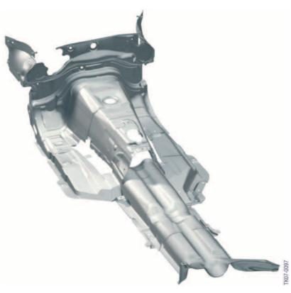
26 - E92 M3 Sound insulating mat and thermal insulation
