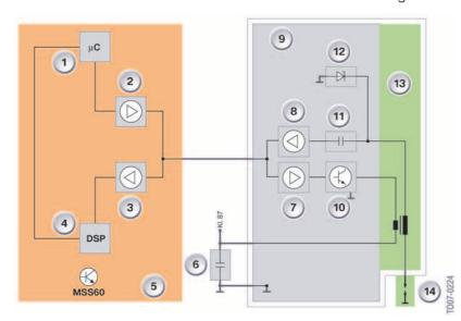
57 - MSS60 Simplified basic layout of ion current monitoring
