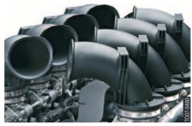
14 - S65B40 Notional view without the intake manifold
