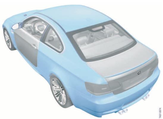
9 - E92 M3 View of M3-specific external body components
