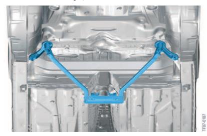
7 - E92 M3 Rear axle braces and transmission tunnel bridge
