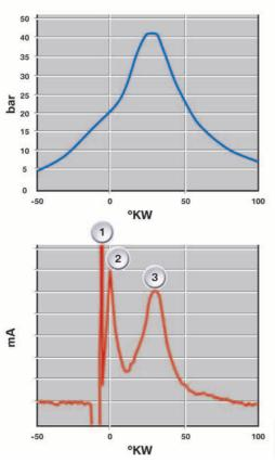
58 - Combustion curve (top) and ionic current (bottom)
