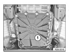
Remove oil drain plug (1). Tightening torque: <u>28 00 3AZ</u>. Drain off transmission oil.
