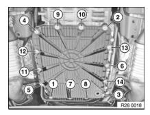
Insert screws until contact with screw heads is made. Screw down to torque in specified sequence (1-14). Tightening torque: <u>28 00 4AZ</u>.
