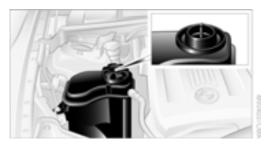
The level indicator 1 in the coolant filler neck indicates the level of coolant. The coolant level is correct when it is between the arrows of the respective inscription on the reservoir **2**.
