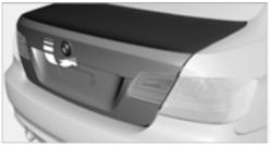
Press the button, see arrow, or the subtrom on the remote control for a longer period. The trunk lid will open slightly. It can now be swung upwards.
