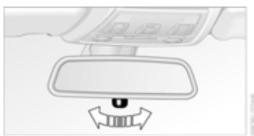
Turn the knob to reduce glare from the headlamps of cars behind you when driving at night.
