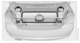
When the hardtop is closed, objects can be placed in the area below and near the cargo area cover.
