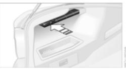
The warning triangle is located on the left-hand side of the trunk. Press the tab to take it out.
