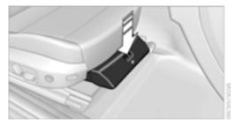
The first aid pouch is located in a compartment under the front passenger seat.
