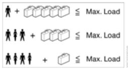
The permissible load is the total of the weight of occupants and cargo/luggage. The greater the weight of the occupants, the less cargo/luggage can be transported.
