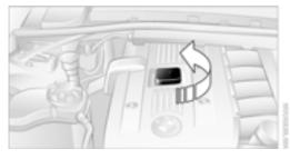
Add up to 1 US guart/1 liter of engine oil only after a corresponding message is shown on the Control Display.
