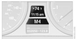
The selector lever position and the engaged gear are displayed, e.g. M4.
