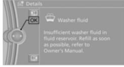
You can call up more information on the Control Display, e.g. on the cause of a malfunction and on how to respond, via Check Control, refer to page 90.
