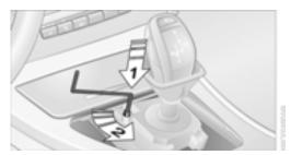
5. Rotate allen wrench until it reaches the stop, arrow **2**. The parking lock is unlocked.
