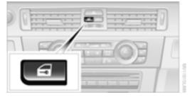
This button serves to unlock or lock doors and the trunk lid when the front doors are unlocked or locked, but does not activate the anti-theft system. Depending on the equipment package, the fuel filler flap can be unlocked as needed.
