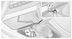
Insert allen wrench into the opening, arrow
