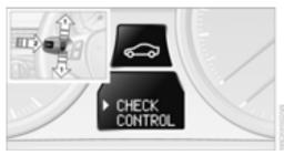
1. Push button 1 in the turn signal/high beam lever up or down repeatedly until the appropriate symbol appears in the display,
