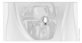
4. Using the screwdriver from the onboard vehicle tool kit, refer to page 262, press the red lever and with the button pressed, simultaneously move the selector lever to the desired position.
