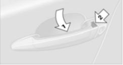
Grasp the handle on the driver's or front passenger door completely, arrow 1. This corresponds to pressing the 🔯 button.
