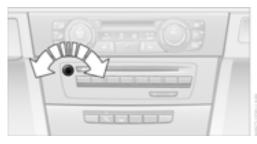
Turn the knob until the desired volume is reached. The setting is stored for the remote control currently in use.
