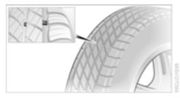
Wear indicators in the base of the tread groove are distributed around the tire's circumference; the letters TWI, for Tread Wear Indicator, on the tire's sidewalls identify tires that incorporate these wear indicators. Once the tire tread has worn down to the wear indicators, the tire has worn to a depth of 0.063 in/1.6 mm.
