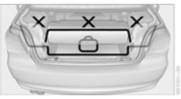
When the hardtop is open, objects can be placed under the cargo area cover. Do not place objects in those areas on the figure that are marked with an X.
