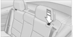
You can fold down the rear seat backrest to transport light objects in the rear without damaging the seats. Depending on the vehicle equipment, the mounting points for the trunk net are found on the rear panel of the backrest. To unlock the rear seat backrest: press the button on the driver's or the opposite side.
