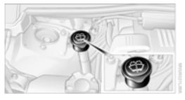
All washer nozzles are supplied with washer fluid by the same reservoir.
