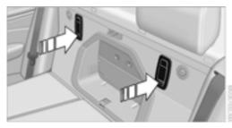
When the rear seat backrest is folded down, you will find two bag holders on the trunk wall:
