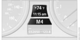
The selector lever position is displayed and, in manual mode, the engaged gear, e.g. M4.
