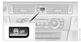
Press the button; the indicator lamp for DSC OFF lights up and TRACTION is displayed in the instrument cluster.
