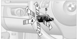
Press the lever upward or downward, arrow 3. The displays on the speedometer disappear.
