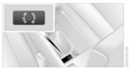
Connection for audio playback: TRS connector 1/8 in/3.5 mm
