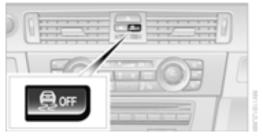
Press the button for at least 3 seconds until the indicator lamp for DSC OFF lights up and DSC OFF is displayed in the instrument cluster. Dynamic Traction Control DTC and DSC have been simultaneously deactivated. Stabilizing and drive-output promoting actions are no longer executed.
