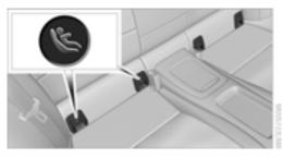
The mounts for the lower LATCH anchors are located behind the labeled protective caps.
