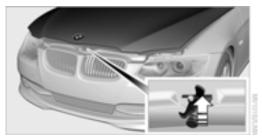
In order to avoid damage, make sure that the wiper arms are against the windshield before you open the hood. Do not open the engine hood before the engine has cooled down; otherwise, injuries may result. Press the release handle and open the hood.
