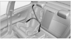
The rear safety belts and the front passenger safety belt can be prevented from being pulled out in order to fasten child restraint systems.
