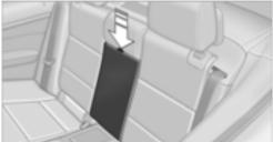
2. Front cover: press the two recesses together and fold the cover down until it engages.
