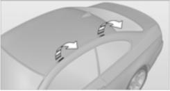
The mounting points are located in the roof.
