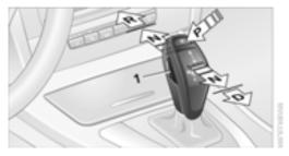
Briefly push the selector lever in the desired direction, overcoming a resistance point if necessary. When shifting out of P or into R, simultaneously press the button **1**.
