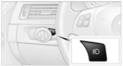
The parking lamps or low beams must be switched on for the fog lamps to operate. The green indicator lamp in the instrument cluster lights up whenever the fog lamps are on.
