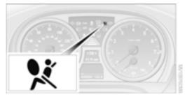
As of radio readiness, refer to page 60, the warning lamp lights up briefly to indicate that the entire airbag system and the belt tensioners are operational.
