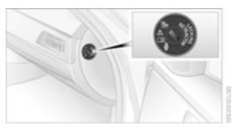
The passenger safety belt can be locked with a key switch so that it is prevented from being pulled out.
