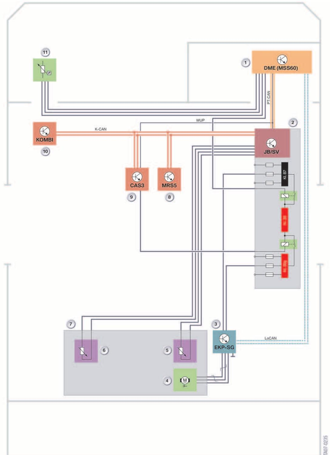
60 - MSS60 Fuel supply system circuit diagram
