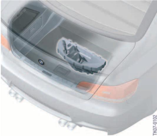
The M3 floor insert in the luggage compartment has been modified to accommodate the M Mobility System.
