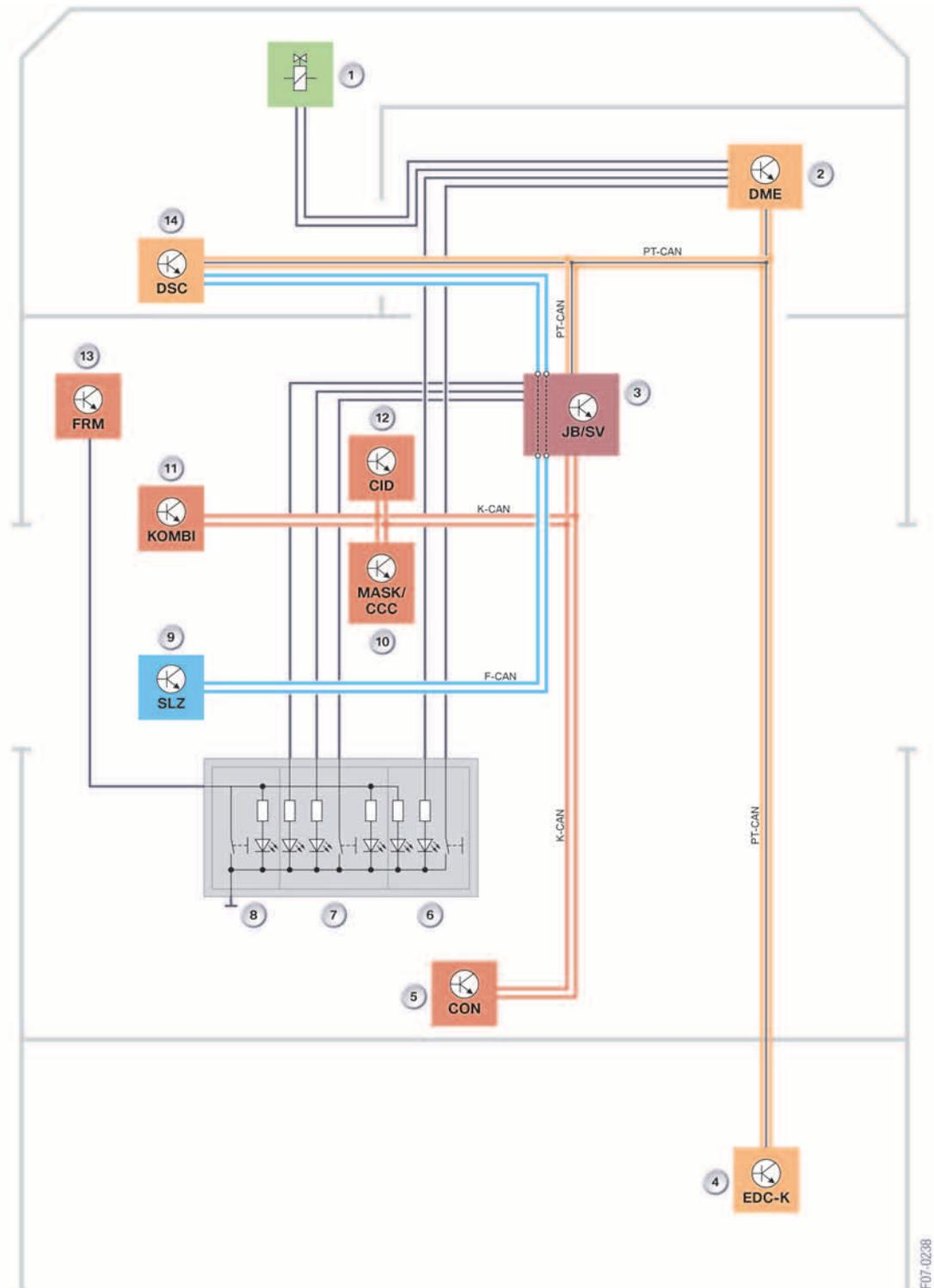
2 - E92 M3 MDrive system circuit diagram
