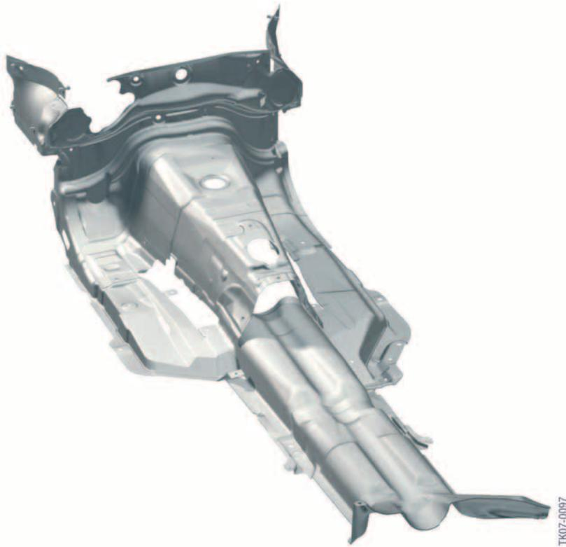
26 - E92 M3 Sound insulating mat and thermal insulation
