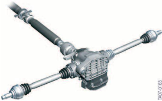
71 - E92 M3 Axle drive with output shafts
