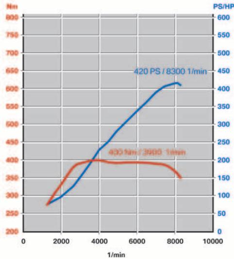
15 - E92 M3: S65B4000 Power and Torque Curve
