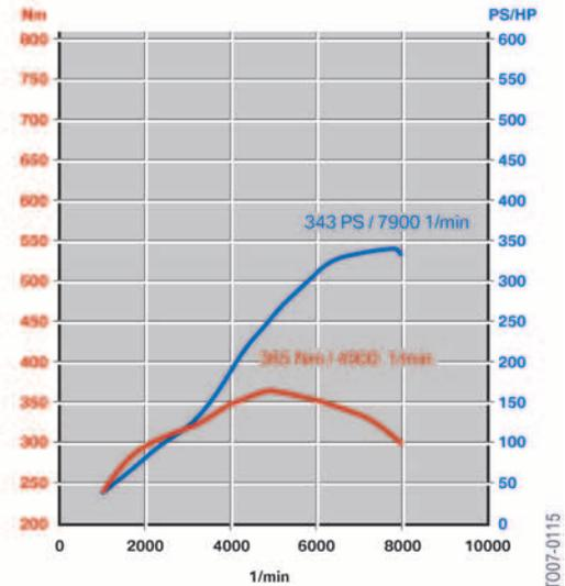
16 - E46 M3: S54B3200 Power and Torque Curve
