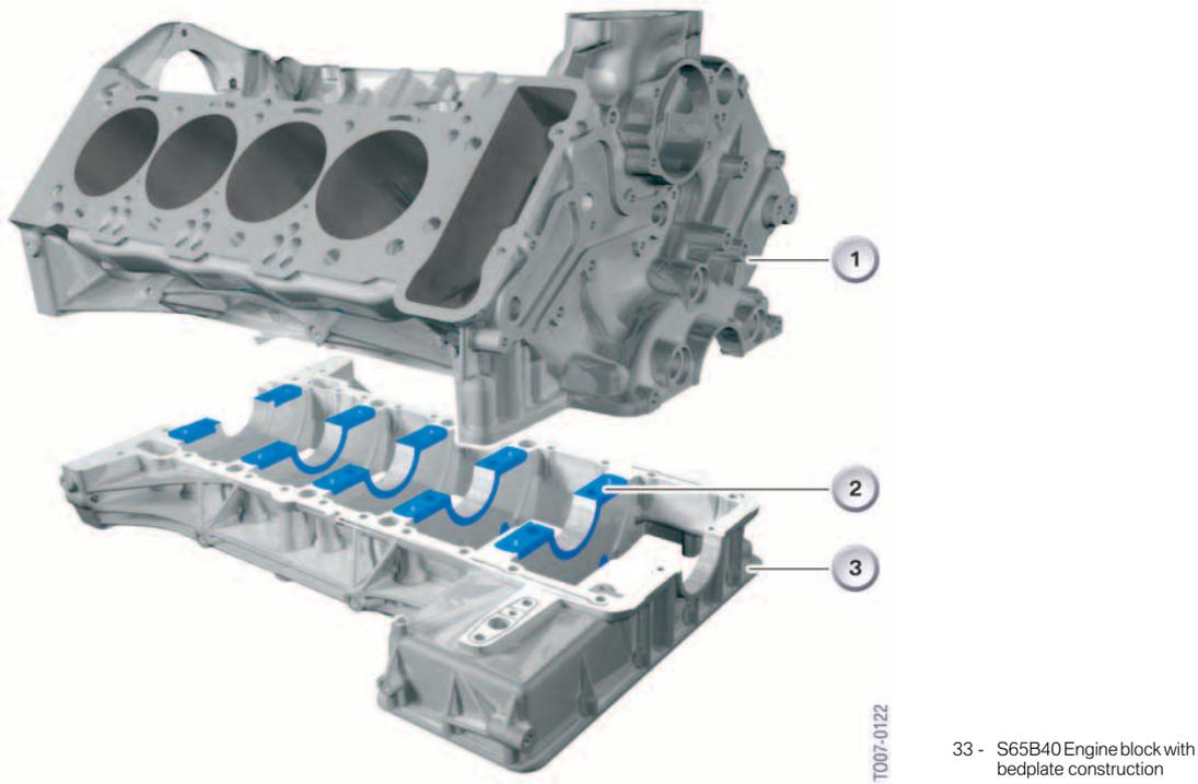
33 - S65B40 Engine block with bedplate construction
