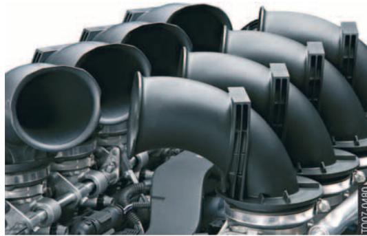
14 - S65B40 Notional view without the intake manifold
