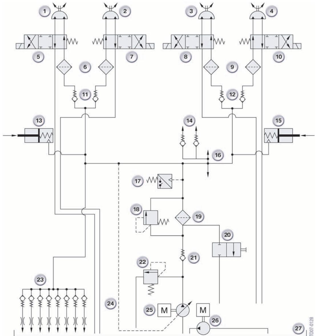
36 - S65B40 Hydraulic schematic of oil supply
