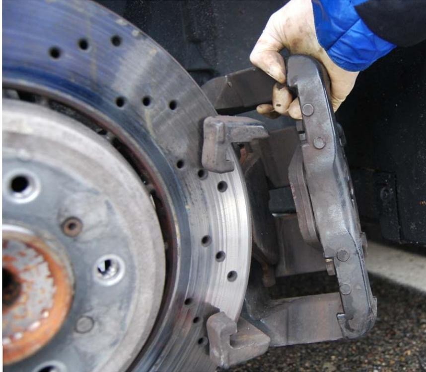
STEP 10. Remove the pads. They are held in the caliper and the piston by springs at this point and will come out when you pull on them. Here, you can see the caliper housing with the
