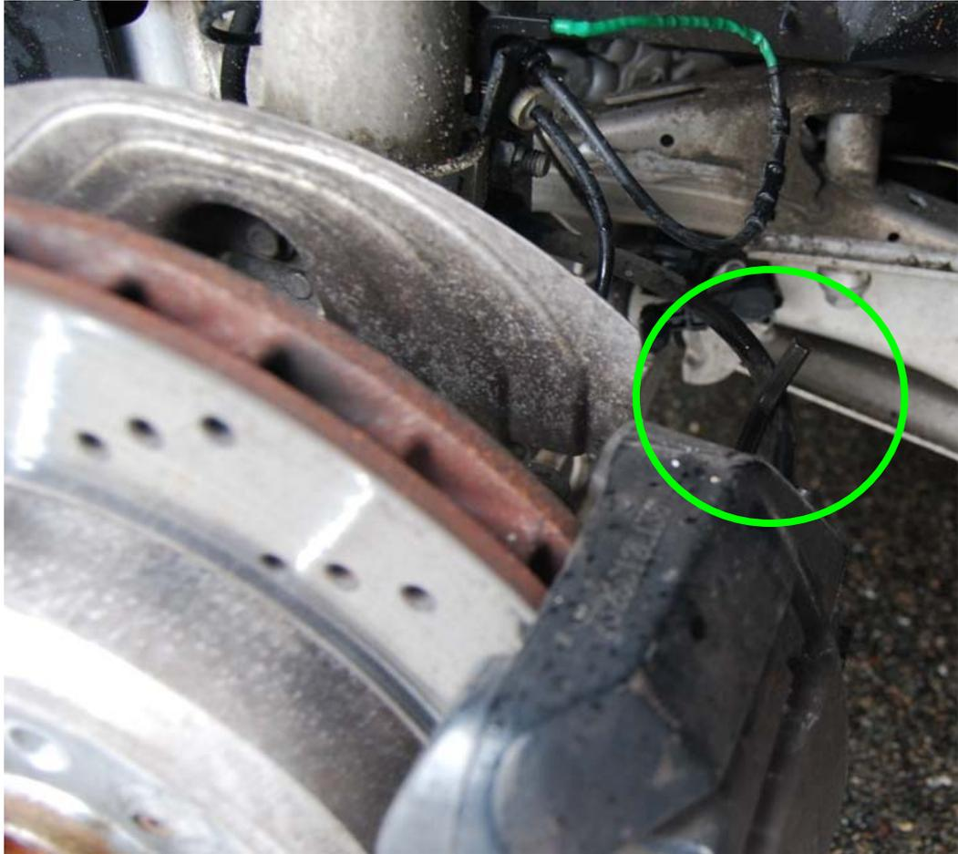
A more detailed view on an allen wrench inserted in to the retaining bolt:
