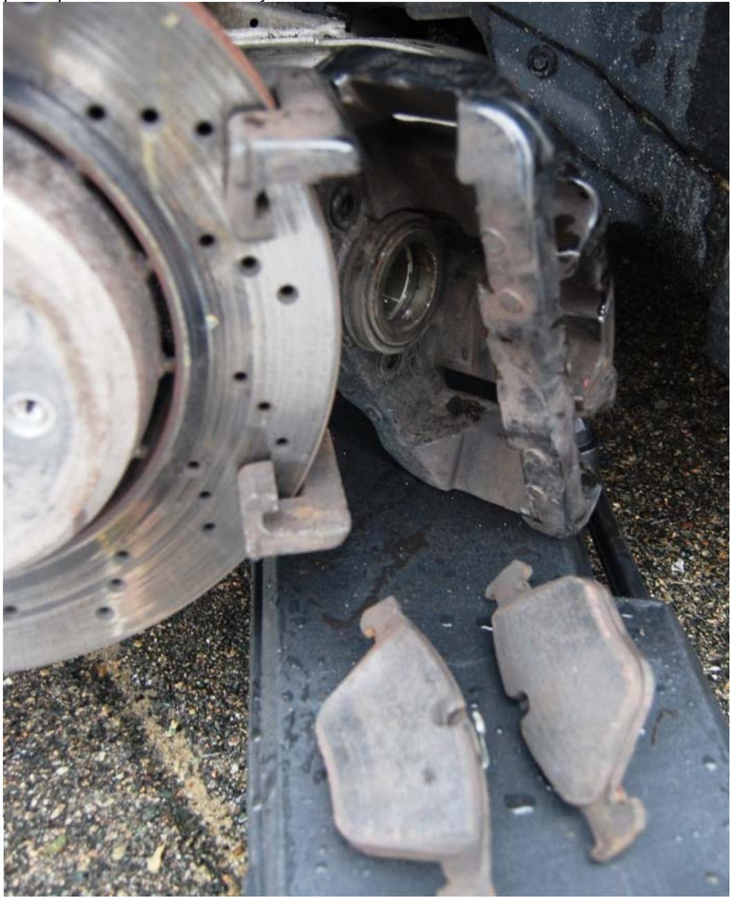
STEP 11. Clip the replacement pads into the piston and the caliper housing.
