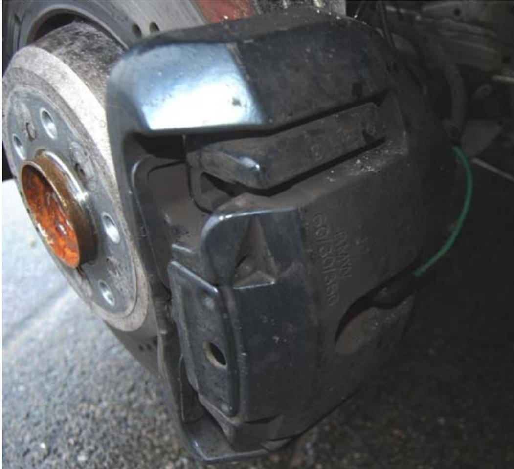
STEP 3. Remove the large anti-rattle spring (#8) using a pair of channel locks or sturdy pliers to pry back one end at a time (I start with the top). If you do this, it should not spring out of place, decreasing risk of injury. Do not use your fingers. Since there is a chance the spring might pop out, wear safety glasses.
