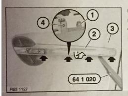
Unlock catches (1) under side panel grille (2) with special tool 64 1 020.
