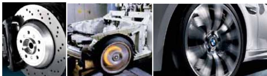
The completely new high-performance compound brake system was specially designed for the BMW M3. Due to its cross-drilled brake disc and partial use of aluminium, it is very lightweight in design. Fully floating, the brake discs can expand freely when stressed to the maximum. The perforations also provide optimum deceleration in wet conditions, on a par with that of ceramic brakes.
