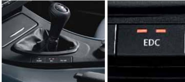
This optional system is unique in this class and offers the most individual customization of suspension settings. With its “Sport”, “Normal” and “Comfort” settings, the EDC system is perfectly matched to the BMW M3.
