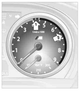
The variable advance warning zone, arrow **1** and arrow **2**, limits the currently permissible engine speed range depending on the engine oil temperature. The permissible engine speed increases as the engine oil temperature rises. If at all possible, avoid engine speeds in the yellow advance warning zone, arrow **1**.
