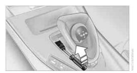
4. Insert the screwdriver into the opening of the white lever, arrow **1**.
