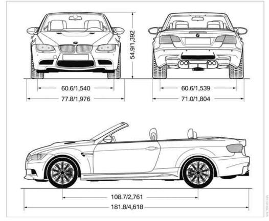
All dimensions given in inches/mm. Smallest turning circle dia.: 38.4 ft/11.7 m.
