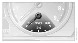
When the engine is at normal operating temperature, the engine oil temperature is between approx.  $175 \degree$ F /80 °C and approx.  $250 \degree$ F /  $120 \degree$ C.
