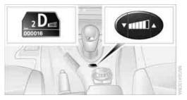
Press the button repeatedly until the desired drive program is displayed in the instrument cluster, refer to page 27.
