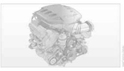
The high-speed V8 engine uses its 244 cu in/ 4 liters of displacement to produce a maximum output of 414 hp and a maximum torque of 295 lb ft/400 Nm. Its spontaneous response results in a very wide effective rpm range. The maximum engine speed is 8,400 rpm and is electronically regulated. Because of the powerful engine dynamics, the maximum engine speed is limited to 7,000 rpm when the vehicle is stationary.
