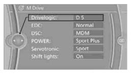
4. Turn the controller to set drive mode or sequential mode.
