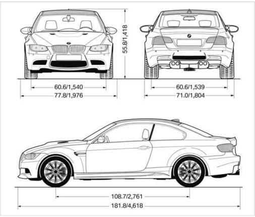
All dimensions given in inches/mm. Smallest turning circle dia.: 38.4 ft/11.7 m.
