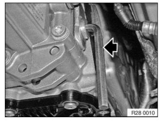
6. Install the filler plug (do not torque it yet).
