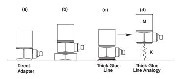
Figure 5: The adhesive mount, direct and with adapter
