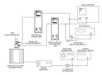
Figure 1: Back-to-back calibration set-up
