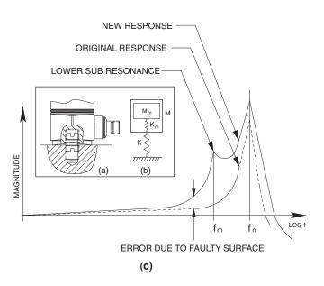
Figure 4: Non-flat accelerometer mounting surface
