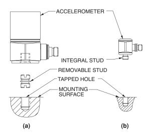
Figure 3: The threaded stud mount
