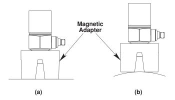
Figure 6: Magnetic mounting adapters
