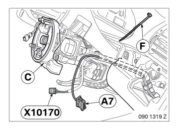
Disconnect all cables from plug **X10170** and connect to branch **A7** as follows:
