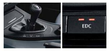
This optional system is unique in this class and offers the most individual customization of suspension settings. With its "Sport", "Normal" and "Comfort" settings, the EDC system is perfectly matched to the BMW M3.
