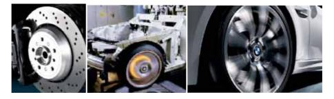
The completely new high-performance compound brake system was specially designed for the BMW M3. Due to its cross-drilled brake disc and partial use of aluminium, it is very lightweight in design. Fully floating, the brake discs can expand freely when stressed to the maximum. The perforations also provide optimum deceleration in wet conditions, on a par with that of ceramic brakes.
